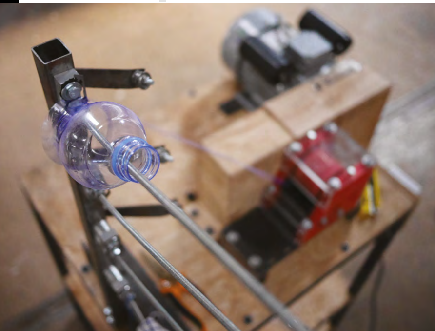
Below ■ The Chopper deconstructing a plastic bottle into even flake
